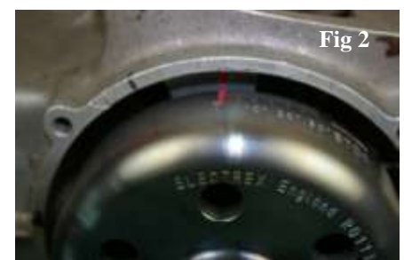
Picture shows ignition only stator, however the position of the lighting stator will be the same
